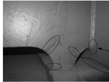
Initiation point of fatigue crack
