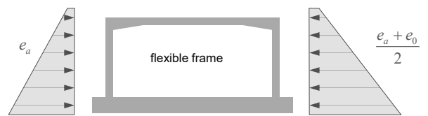
Earth pressure transfer in closed frame bridge (underpass)
