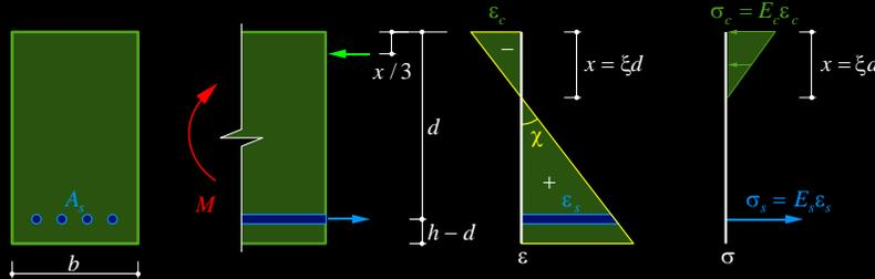
$$\text{Spannungen: } \sigma_s = \frac{M}{A_s \left( d - \frac{x}{3} \right)} = \frac{M}{bd^2} \frac{1}{\rho \cdot \left( 1 - \frac{\xi}{3} \right)}, \quad \sigma_c = \frac{2 \cdot M}{b \cdot x \cdot \left( d - \frac{x}{3} \right)} = \frac{M}{bd^2} \frac{2}{\xi \left( 1 - \frac{\xi}{3} \right)} \left( = \frac{\sigma_s}{n} \cdot \frac{\xi}{1 - \xi} \right)$$
