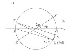
$$\begin{split} &\sigma_n = \sigma_x \cos^2 \phi + \sigma_z \sin^2 \phi + 2\tau_{xz} \sin \phi \cos \phi \\ &\sigma_t = \sigma_x \sin^2 \phi + \sigma_z \cos^2 \phi - 2\tau_{xz} \sin \phi \cos \phi \\ &\tau_{nt} = (\sigma_z - \sigma_x) \sin \phi \cos \phi + \tau_{xz} (\cos^2 \phi - \sin^2 \phi) \end{split}$$
