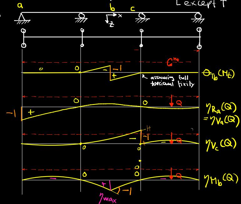
Based on the IL, the governing load arrangement can be found, e.g. for the max. bending moment in b (IL shown at bottom,  $\gamma_{M_b}(Q)$ ), considering rail traffic LMI:
