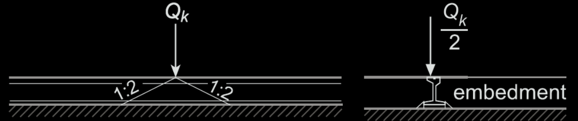
Grooved rail embedded in concrete
