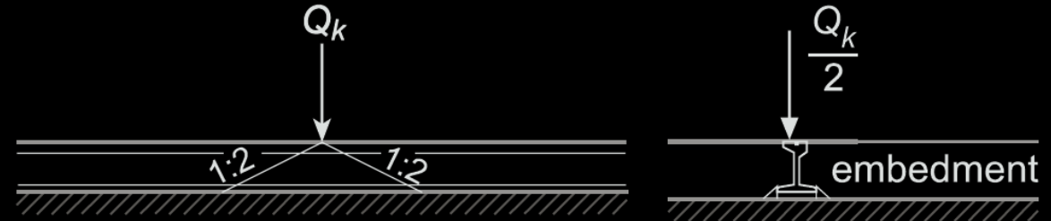
Grooved rail embedded in concrete
