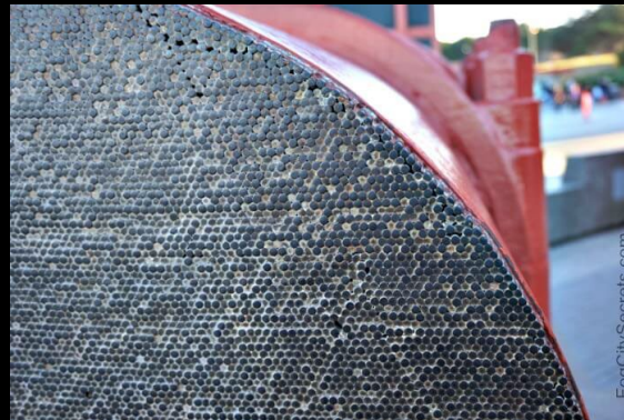
Cable detail (note outermost wires deformed by compaction)
