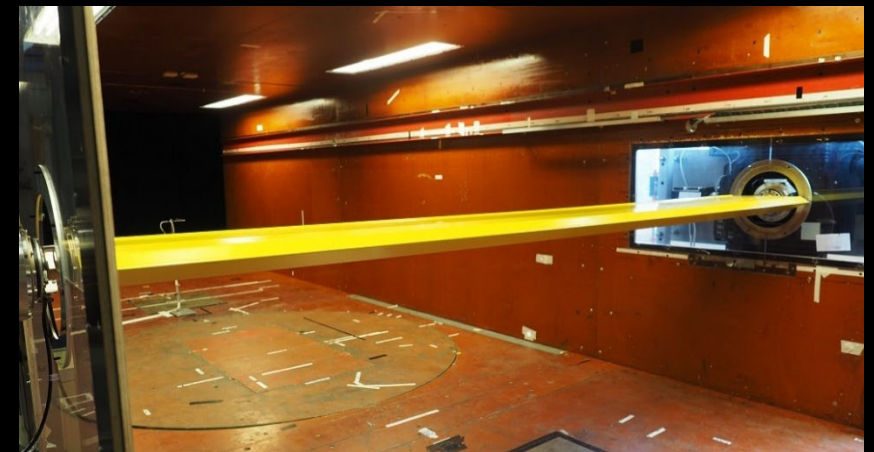
Wind tunnel test of a bridge section at NTNU
