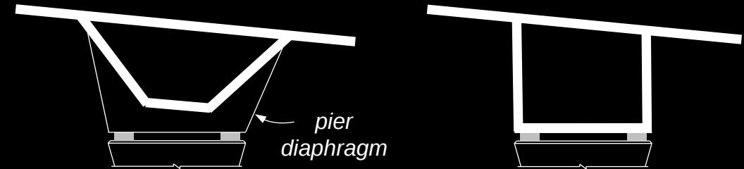
Superelevation Treatment Alternatives
