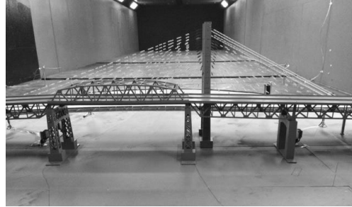
Wind tunnel testing on a new cable-stayed bridge; the presence of an existing truss bridge is accounted for, in order to capture potential interaction between the bridges.
