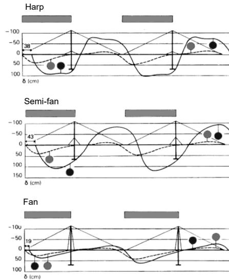
*Asymmetric LL causes longitudinal deck displacement*
