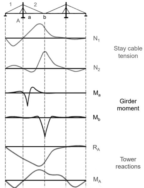
Note that the above influence lines correspond to the typical arrangement where the towers are stabilised through backstays and anchor piers.
