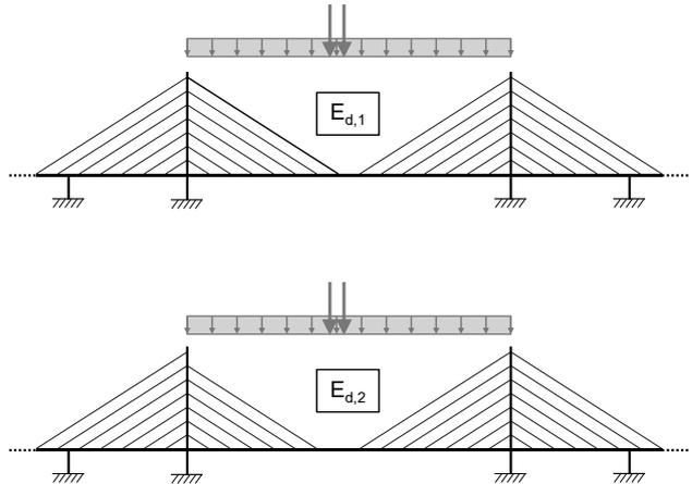
Note that the requirement of the Eurocode approach to apply the same live load on both systems can be challenging. This is because if generated by influence lines, the governing load pattern will be different for the two systems. Therefore, one must capture the governing load pattern for the intact system and manually apply that pattern to the system with the removed cable.
