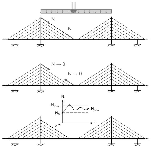
$N_0$  = Initial axial force in cable under consideration prior to cable loss
