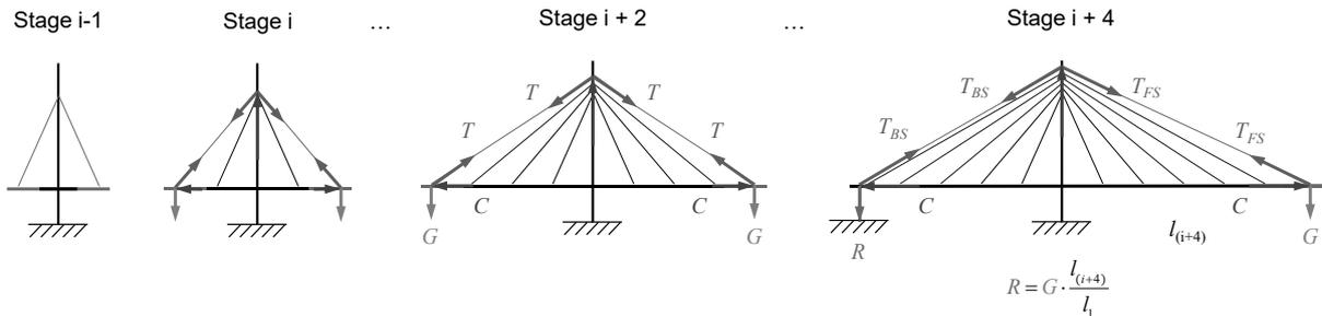
During the erection stages when girder and deck segments are installed symmetrically about the tower, the stay cable forces (and corresponding compressive forces in the superstructure) can be calculated by considering force equilibrium at the deck level (see illustrated Stages i and i+2).
