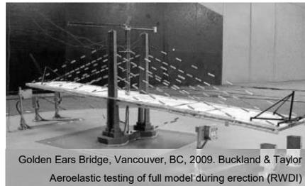
In general, steel composite superstructures are more sensitive to wind loading than concrete superstructures (mass helps – see Chapter 9.1: Common Aspects).
