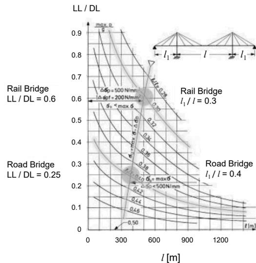
A side span to main span ratio of less than 0.5 allows for tensioning of the backstays and results in a stiffer structure.
