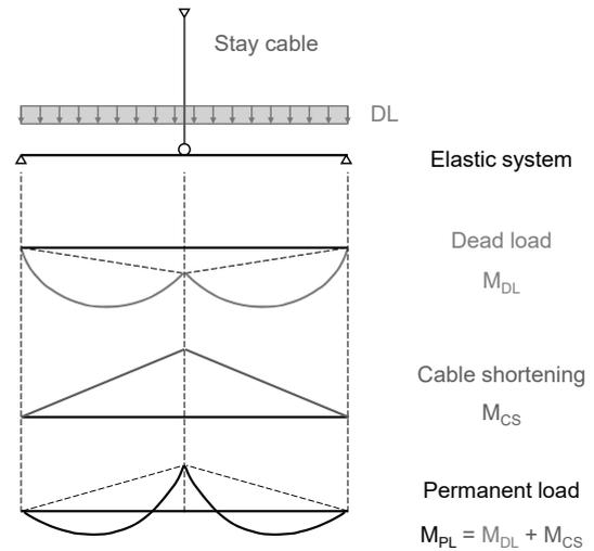
Considering the simple case of a propped beam, it can be seen how the final bending moment diagram under permanent loads can be adjusted by imposing appropriate cable shortening.
