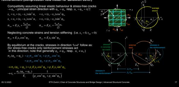
Derivation of the factor for deviation of the principal direction  $\varphi_0$  of the shear force from the direction of the principal reinforcement (compression field model for sandwich cover)
