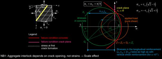
NB2: The load-bearing capacity due to aggregate interlock is not necessarily sufficient in regions subjected to high shear stress (slabs in the support area) to avoid brittle failure in the event of initial shear cracking!
