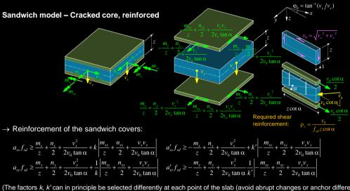
(The factors *k*, *k*' can in principle be selected differently at each point of the slab (avoid abrupt changes or anchor differential reinforcement forces). Selection of the compression field inclination  $\alpha$ : Analogous considerations as with beams. (Often  $k = k' = \cot \alpha = 1$  is chosen.)
