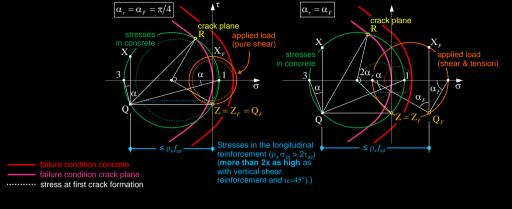
NB: There is a scale effect and the validity is limited to moderate shear stresses!
