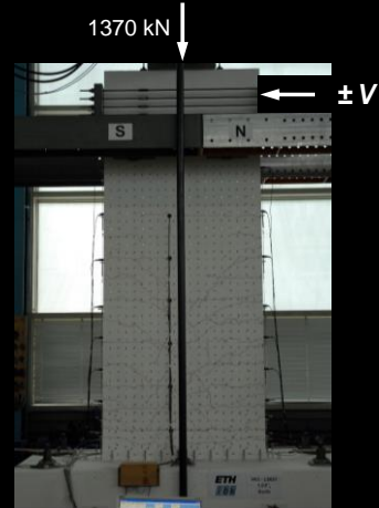
VK1: first yielding of reinforcement
