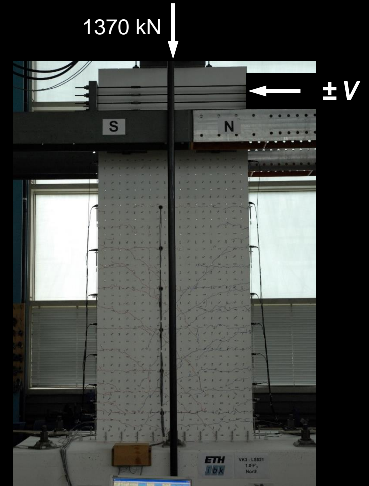
VK1: first yielding of reinforcement
