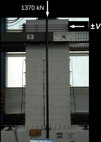
VK1: first yielding of reinforcement
