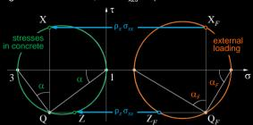
x, z: directions of reinforcement, behaviour not isotropic (also not for  $a_{sx} = asz$ )!
