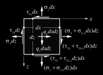
A stress component is taken as positive if it acts in a positive (negative) direction on an element face where a vector normal to the face is in a positive (negative) direction relative to the axis considered.
