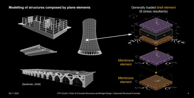
Most concrete structures can be modelled as a superposition of local plane elements. A plane element subjected to general loading can be modelled by a combination of membrane elements. This general loading can be modelled as sublayers subjected to in-plane loads (membrane elements).
