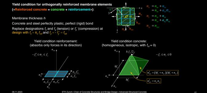
Repetition Stahlbeton I: Yield conditions of orthogonally reinforced membrane elements:
