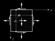
The local behaviour of a plane structure subjected to a general loading (i.e. in-plane forces, bending moments, twisting moments, and transverse shear) can be modelled by a combination of membrane elements (sandwich or layered approaches). With numerical approaches, the behaviour of most structures can be modelled by the superposition of membrane elements (see the following slide).
