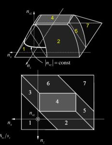
SN: Reinforcement areas per unit length in x- and z-direction  $a_{xx} = A_{xx}/s_x$   $a_{xz} = A_{xz}/s_z$
