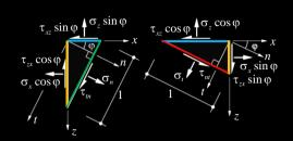
$$\begin{split} \sigma_n &= \frac{\sigma_x + \sigma_z}{2} + \frac{\sigma_x - \sigma_z}{2} \cos 2\phi + \tau_{xz} \sin 2\phi \\ \sigma_t &= \frac{\sigma_x + \sigma_z}{2} + \frac{\sigma_x - \sigma_z}{2} \cos 2\phi - \tau_{xz} \sin 2\phi \\ \tau_m &= -\frac{\sigma_x - \sigma_z}{2} \sin 2\phi + \tau_{xz} \cos 2\phi \end{split}$$
