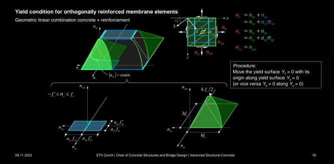
Repetition Stahlbeton I: Yield conditions of orthogonally reinforced membrane elements
