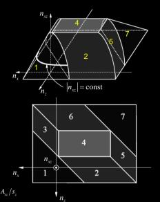
SN: Reinforcement areas per unit length in x- and z-direction  $a_{_{\rm xx}}=A_{_{\rm xx}}/s_{_{\rm x}}$   $a_{_{\rm zz}}=A_{_{\rm zz}}/s_{_{\rm z}}$
