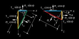
$$\begin{split} \sigma_{n} &= \frac{\sigma_{x} + \sigma_{z}}{2} + \frac{\sigma_{x} - \sigma_{z}}{2} \cos 2\phi + \tau_{xz} \sin 2\phi \\ \sigma_{r} &= \frac{\sigma_{x} + \sigma_{z}}{2} + \frac{\sigma_{x} - \sigma_{z}}{2} \cos 2\phi - \tau_{xz} \sin 2\phi \\ \tau_{m} &= -\frac{\sigma_{x} - \sigma_{z}}{2} \sin 2\phi + \tau_{xz} \cos 2\phi \end{split}$$
