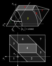
SN: failure type: very ductile / ductile (except for very flat stress field inclinations) / brittle  $^{1}n_{z}$
