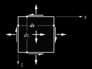
The local behaviour of a plane structure subjected to a general loading (i.e. in-plane forces, bending moments, twisting moments and transverse shear) can be modelled by a combination of membrane elements (sandwich or layered approaches). With numerical approaches, the behaviour of most structures can be modelled by the superposition of membrane elements (see following slide).
