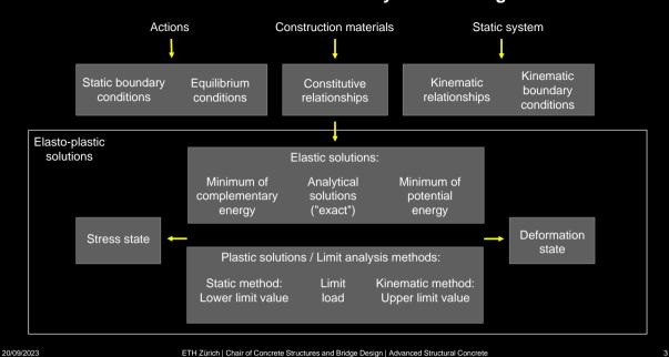
The figure shows the different design methods for concrete structures. In many cases limit analysis methods (plastic solutions) are used, while often implicitly.
