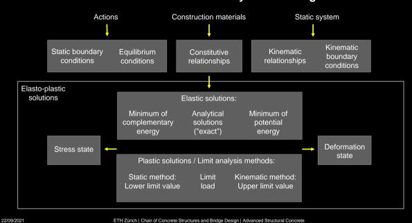
The figure shows the different design methods for concrete structures. In many cases limit analysis methods (plastic solutions) are used, while often implicitly.
