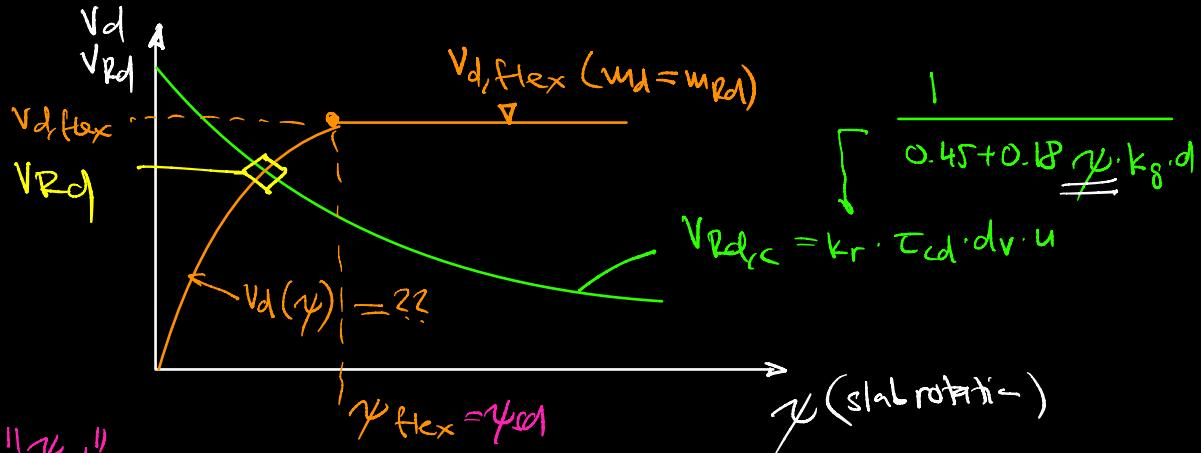
$$\chi = \left[ \frac{\psi_{sd}}{1.5 \cdot \frac{r_s}{c} \frac{f_{sd}}{E_{sd}}} \left( \frac{m_{sd}}{m_{Rd}} \right)^{3/2} \right] = \psi_{sd} \left( \frac{m_{sd}}{m_{Rd}} \right)^{3/2}; \frac{\psi}{\psi_{sd}} = \left( \frac{m_{sd}}{m_{Rd}} \right)^{3/2} \quad \square^{2/3}$$
