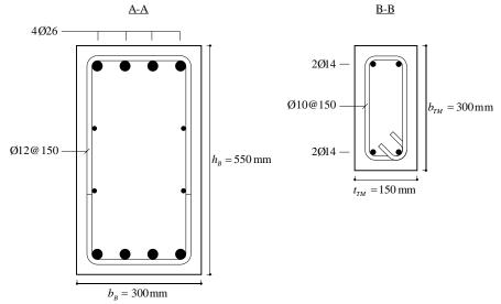
**Material Properites**  $f_{cd} = 16.5 \,\mathrm{MPa}; \, f_{cm} = 33 \,\mathrm{MPa}$ Concrete C25/30 Table 8 and 3  $\varepsilon_{cud} = 0.3\%$ 3.1.2.3.3  $E_{\rm cm} = k_e \sqrt[3]{f_{\rm cm}} \approx 30.1 \text{GPa}$ Table 3  $f_{ctm} = 2.6 \,\mathrm{MPa}$  $f_s = 500 \,\text{MPa}; f_{sd} = 435 \,\text{MPa}; f_t = 540 \,\text{MPa}$ Steel B500B Table 5 and 9
