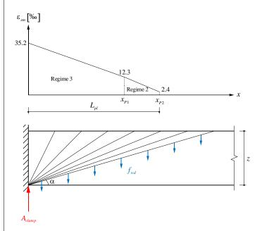
The strain distribution of the reinforcement is assumed as linear within regime 2 and 3.
