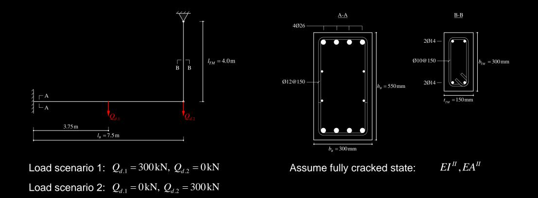
Task: Verify bearing capacity of the structure considering the deformation demand and the deformation capacity
