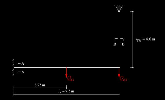
Load scenario 1:  $Q_{d.1} = 300 \text{ kN}, Q_{d.2} = 0 \text{ kN}$ Load scenario 2:  $Q_{d.1} = 0 \text{ kN}, Q_{d.2} = 300 \text{ kN}$
