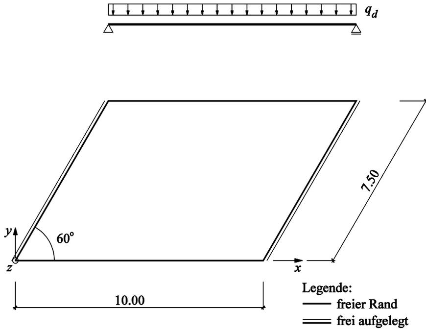
**A2 Results of a FEM-Calculation for a skew-supported slab**
