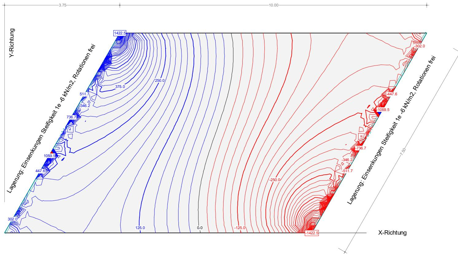
A2.6 Internal force  $v_y$  in [kN/m] resulting from reference load  $p = -100 \text{ kN/m}^2$ , contour lines at 25 kNm/m, dimensions in [m]
