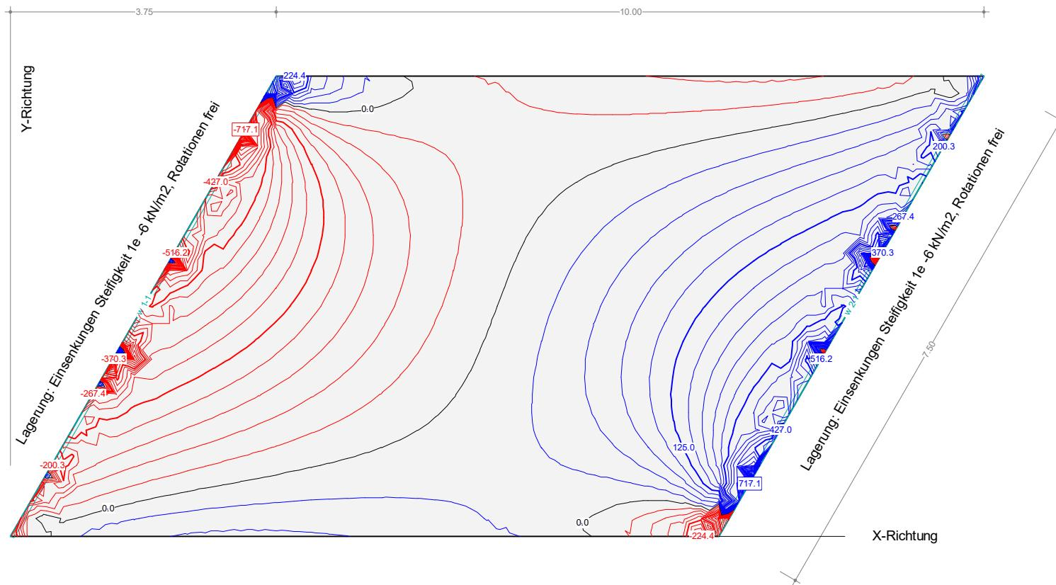
A2.7 Support reaction in [kN/m] resulting from reference load  $p = -100 \text{ kN/m}^2$ , averaged in parts, dimensions in [m]
