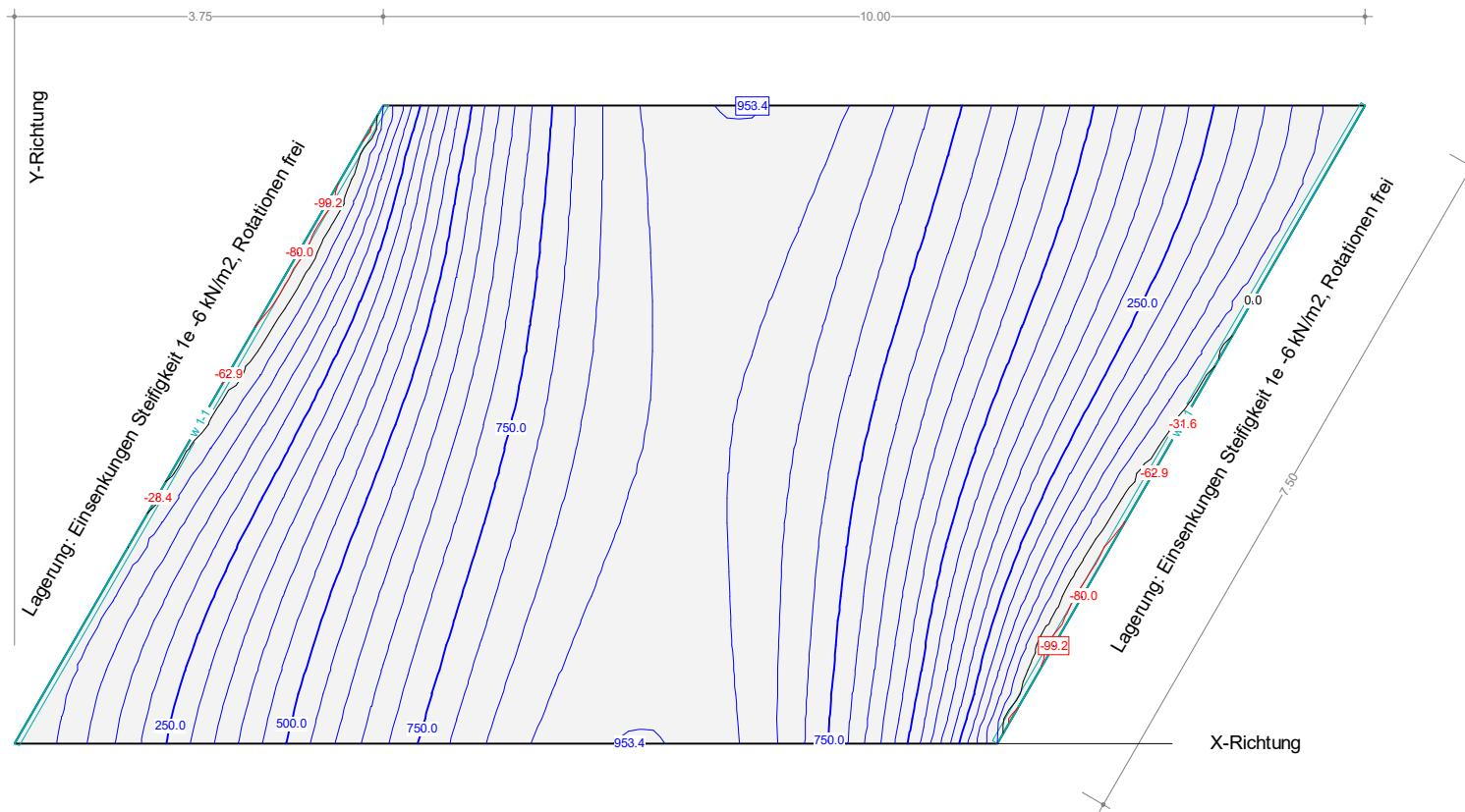
A2.3 Internal force  $m_y$  in [kNm/m] resulting from reference load  $p = -100 \text{ kN/m}^2$ , contour lines at 20 kNm/m, dimensions in [m]
