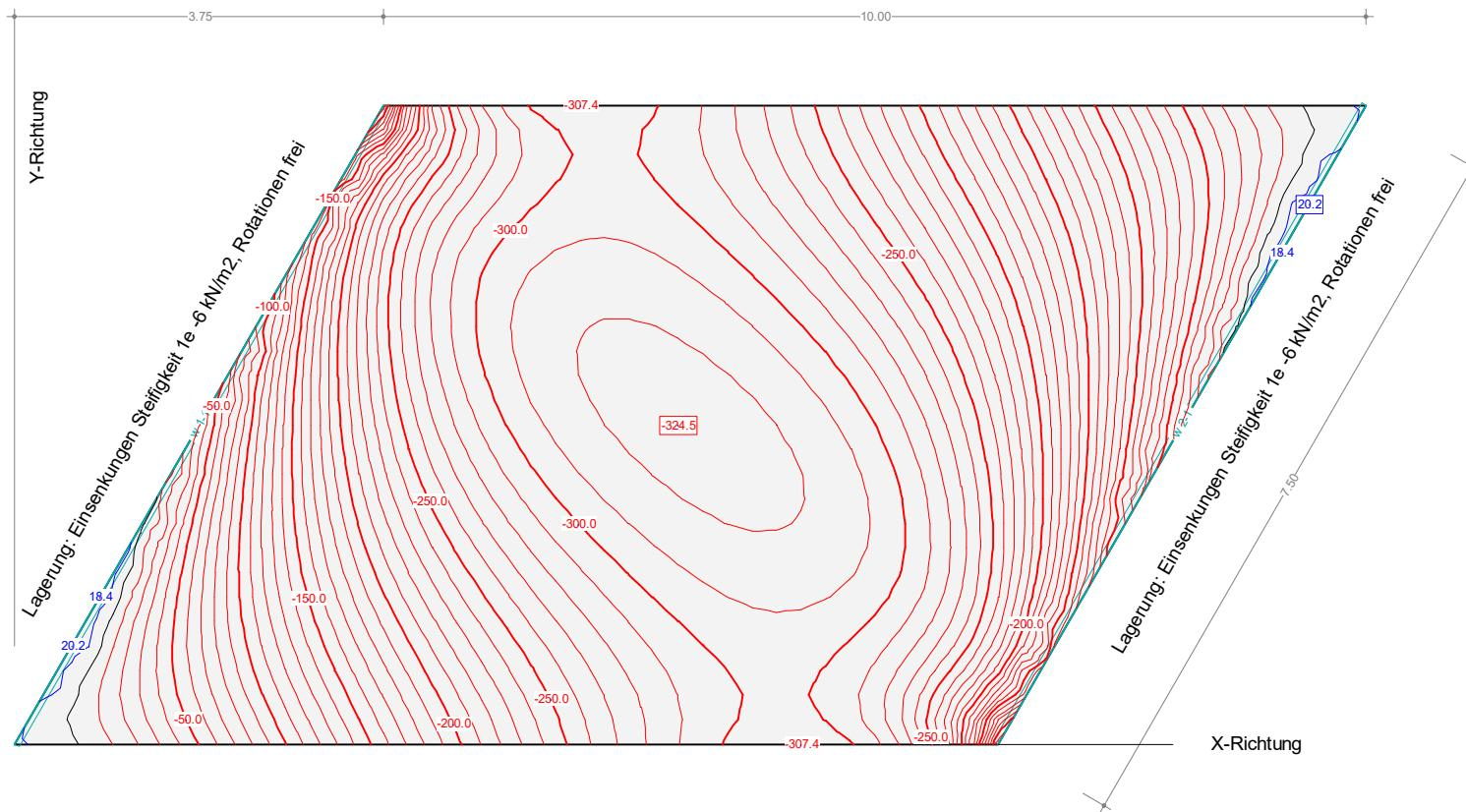
A2.5 Internal force  $v_x$  in [kN/m] resulting from reference load  $p = -100 \text{ kN/m}^2$ , contour lines at 25 kNm/m, dimensions in [m]
