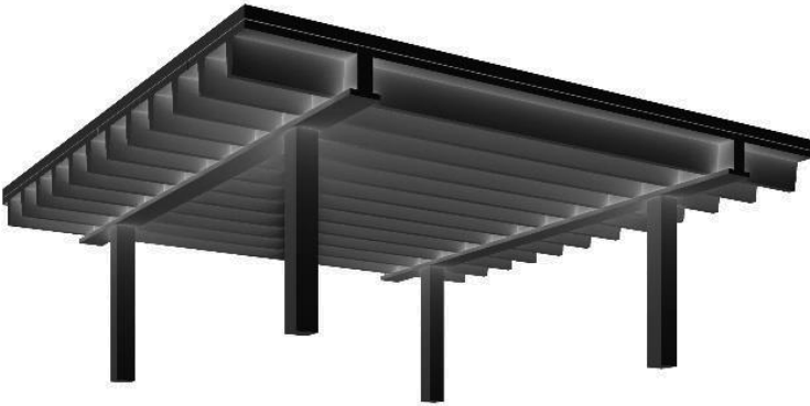
Ribbed slab (with topping)
