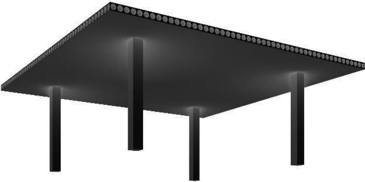
Voided flat slab
