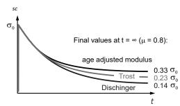
The Trost method is simple and agrees well with experiments (better than more complicated procedures) → only this procedure is used in the following!
