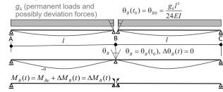
$$M_B(t_0) = M_{Be} = 0, \quad \theta_B(t_0) = \theta_{B0} = \frac{g_k l^3}{24EI}$$
