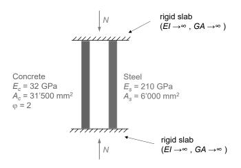
How is the load *N* distributed between the two columns?
