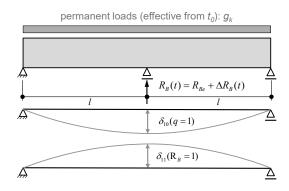
ightarrow Generalization to general systems is possible ightarrow With uniform creep properties, the redundant variables of stat. indeterminate systems do not change!
