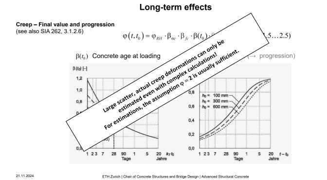
Creep and relaxation are subject to similarly large scatter as shrinkage (5% fractile values of the creep coefficient are  $\pm$  30...40% in experiments).
