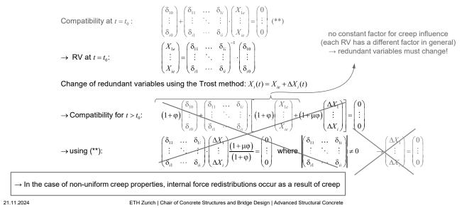
The comparison with the *n*-fold statically indeterminate system with the same creep properties shows that redistributions are required in case of non-uniform creep properties.
