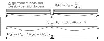
As a general rule, in system changes, creep largely builds up the stress state of the system built in one casting  $\sigma_{OC}$ . The higher the creep coefficient, the closer it approximates the state of the system built in one casting («Einguss-System» in German).
