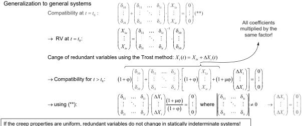
i the creep properties are uniform, redundant variables do not change in statically indeterminate systems:
