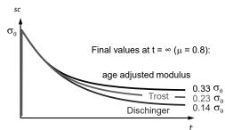
The Trost method is simple and agrees well with experiments (better than more complicated procedures)  $\rightarrow$  only this procedure is used in the following!
