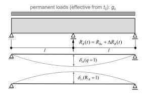
$\rightarrow$  Generalization to general systems is possible  $\rightarrow$  With uniform creep properties, the redundant variables of stat. indeterminate systems do not change!
