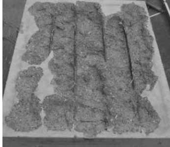
Continuous spalling after 17 min of fire exposure d_p = 0 mm
