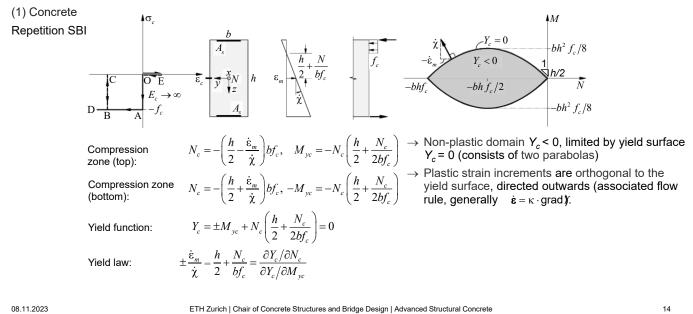
Repetition Stahlbeton I (or Baustatik): Bending and normal force
