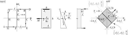
→ Non-plastic domain  $Y_s < 0$  for two reinforcement layers is a parallelogram (for symmetrical reinforcement  $A_s = A'_s \rightarrow$  rhombus), which is defined by the vectors corresponding to the two reinforcement layers.
