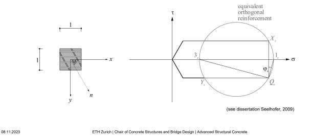
The stress state of the concrete and the reinforcement are in equilibrium with the applied stresses.
