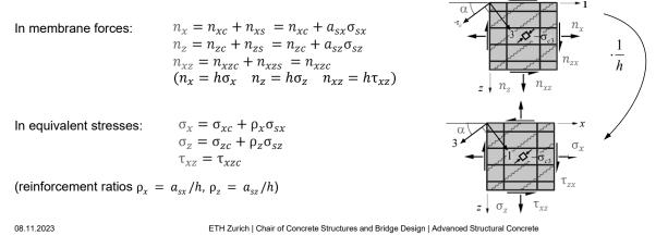
Repetition Stahlbeton I: Forces in orthogonally reinforced membrane elements
