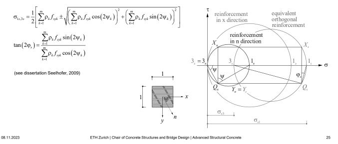
The following slides show how skew reinforcements can be designed and how the corresponding yield conditions can be determined [Seelhofer (2009)]. By the term "skew reinforcement", we refer here to oblique reinforcement directions (as opposed to orthogonal reinforcement), and NOT to orthogonal reinforcement simply rotated with respect to the coordinate axes, as it is sometimes called "skew reinforcement" in literature.
