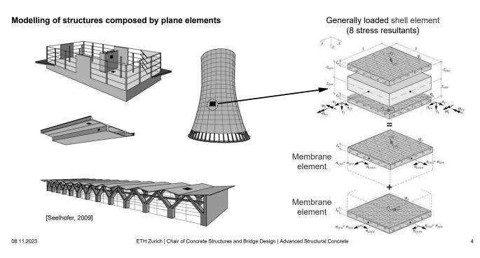
Most concrete structures can be modelled as a superposition of local plane elements. A plane element subjected to general loading can be modelled by a combination of membrane elements. This general loading can be modelled as sublayers subjected to in-plane loads (membrane elements).
