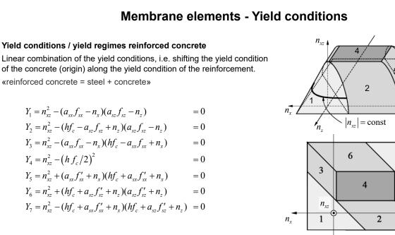
SN: Reinforcement areas per unit length in x- and z-direction  $a_{sx} = A_{sx}/s_x$   $a_{sz} = A_{sz}/s_z$
