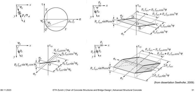
Similarly to orthogonal reinforcement, the yield conditions of membrane elements reinforced in a number of arbitrary directions can also be determined by a graphical linear combination of the non-plastic zones of concrete and reinforcement.
