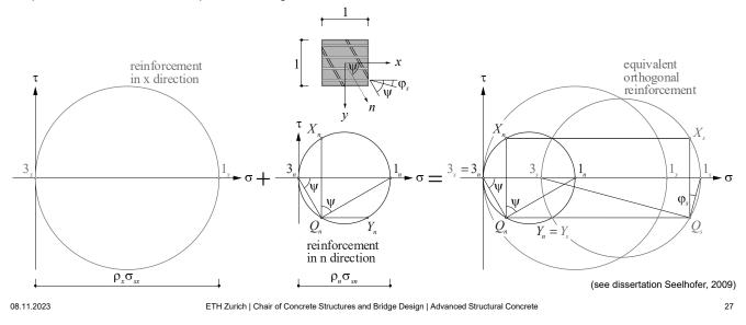
To obtain the equivalent orthogonal reinforcement, the reinforcements in x- and n-direction are superimposed. In contrast to the reinforcement in the x-direction, the inclined reinforcement (n-direction) has a shear component.
