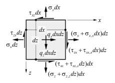
A stress component is taken as positive if it acts in a positive (negative) direction on an element face where a vector normal to the face is in a positive (negative) direction relative to the axis considered.
