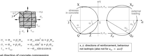
Representation with Mohr's circles (straightforward for orthogonal reinforcement, since  $\tau_{xzs} = 0$ ):
