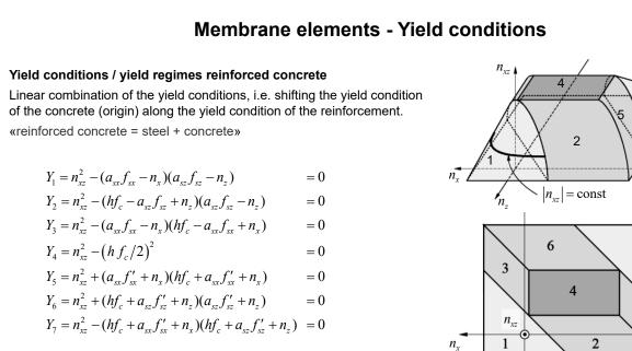
SN: Reinforcement areas per unit length in x- and z-direction  $a_{sx} = A_{sx}/s_x$   $a_{sz} = A_{sz}/s_z$
