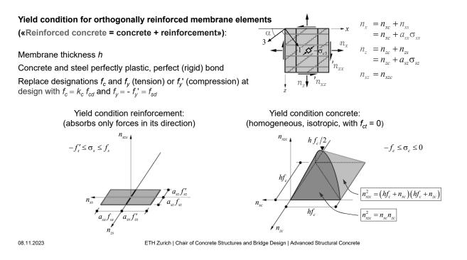
Repetition Stahlbeton I: Yield conditions of orthogonally reinforced membrane elements:
