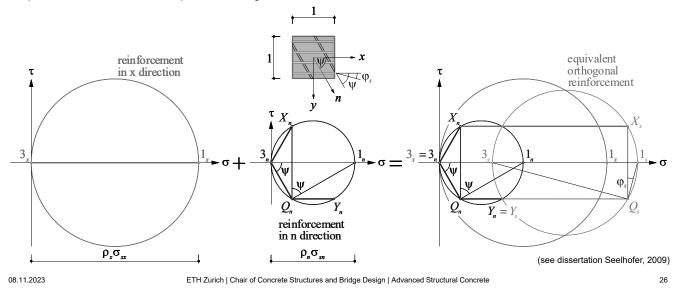
To obtain the equivalent orthogonal reinforcement, the reinforcements in x- and n-direction are superimposed. In contrast to the reinforcement in x-direction, the inclined reinforcement (n-direction) has a shear component.
