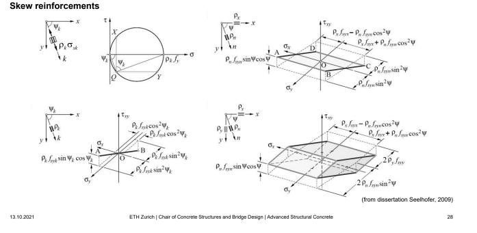
Similarly to orthogonal reinforcement, the yield conditions of membrane elements reinforced in a number of arbitrary directions can also be determined by a graphical linear combination of the non-plastic zones of concrete and reinforcement.
