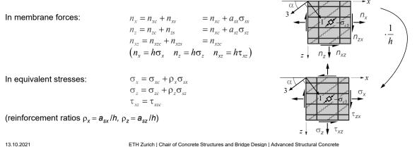
Repetition Stahlbeton I: Forces in orthogonally reinforced membrane elements
