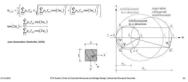
The following slides show how skew reinforcements can be designed and how the corresponding yield conditions can be determined [Seelhofer (2009)]. By the term "skew reinforcement", we refer here to oblique reinforcement directions (as opposed to orthogonal reinforcement), and NOT to orthogonal reinforcement simply rotated with respect to the coordinate axes, as sometimes called "skew reinforcement" in literature.
