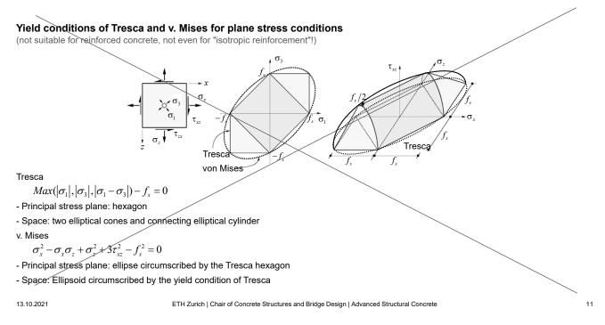
Yield conditions for isotropic materials (e.g. steel: Tresca, von Mises) cannot be applied to reinforced concrete, neither for the dimensioning of reinforcement and not even if it is "isotropic" (equal reinforcement ratio in both directions). Their application can be on the safe or unsafe side.
