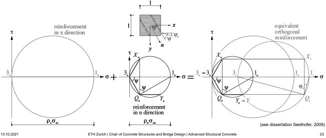
Graphical determination of the equivalent orthogonal reinforcement
