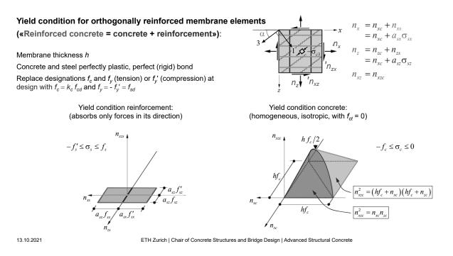
Repetition Stahlbeton I: Yield conditions of orthogonally reinforced membrane elements:
