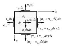
A stress component is taken as positive if it acts in a positive (negative) direction on an element face where a vector normal to the face is in a positive (negative) direction relative to the axis considered. Positive membrane forces correspond to positive stresses Indices: 1-direction of the stress, 2-direction of the normal vector Equilibrium in directions *x*, *z*:
