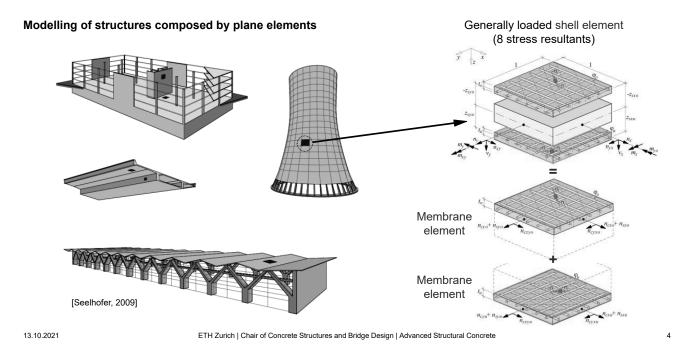
Most concrete structures can be modelled as a superposition of local plane elements. A plane elements subjected to general loading can be modelled by a combination of membrane elements. This general loading can be modelled as sublayers subjected to in-plane loads (membrane elements).
