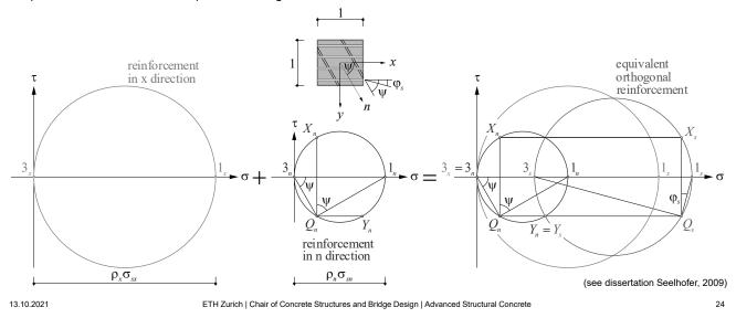
Graphical determination of the equivalent orthogonal reinforcement
