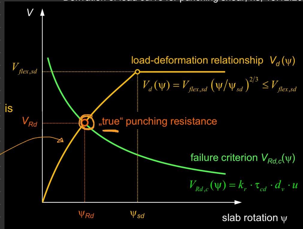
$V_{flex, sd}$  Support reaction at which the bending reinforcement yields (in the considered direction)
